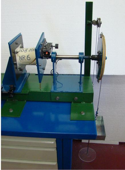
Fig 8. The set-up for the torsion test after the failure of the specimen
